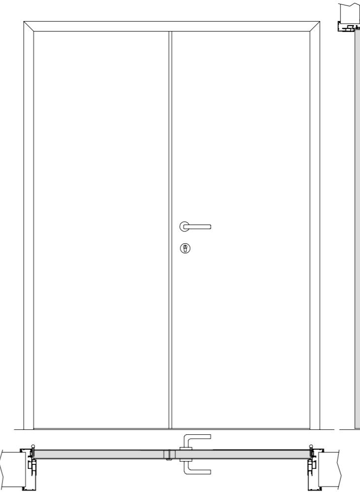
**EN Technical Information.** Doors in panels of phenolic compact sandwich (EPS coated with phenolic 3 or 4mm) with thickness 38mm. Aluminum telescopic frame and stainless steel hardware, including: hinges, lock or free/occupied lock and handle.
